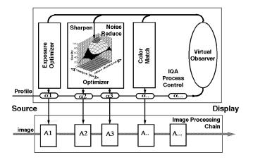
Figure 1. IQA architecture: A, represent Image processing filters in the image processing chain;  $\alpha_i$  represent algebraic models of the Image processing filters in the image processing chain.
