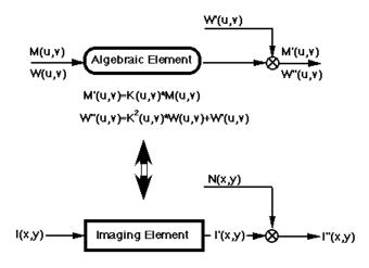
Figure 2. Linear stationary model of Imaging element as implemented in IQA Process Control.
